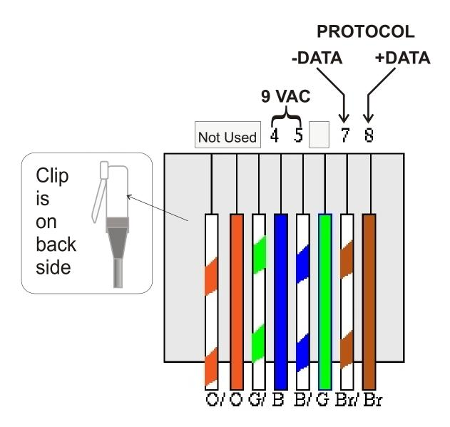
PROTOCOL bus connection using RJ45/CAT5 Cable
