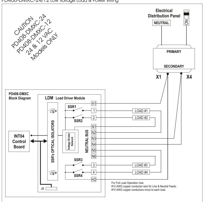
Figure 6 - PD408-DMXC-12/24 **Typical Low Voltage Wiring.**
