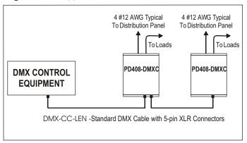
Figure 1 - PD408-DMXC Functional Block Diagram
