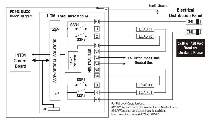
Figure 4. PD408-DMXC Typical 120 VAC Wiring.
