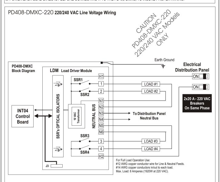
Figure 5. PD408-DMXC-220 Typical 220 VAC Wiring.
