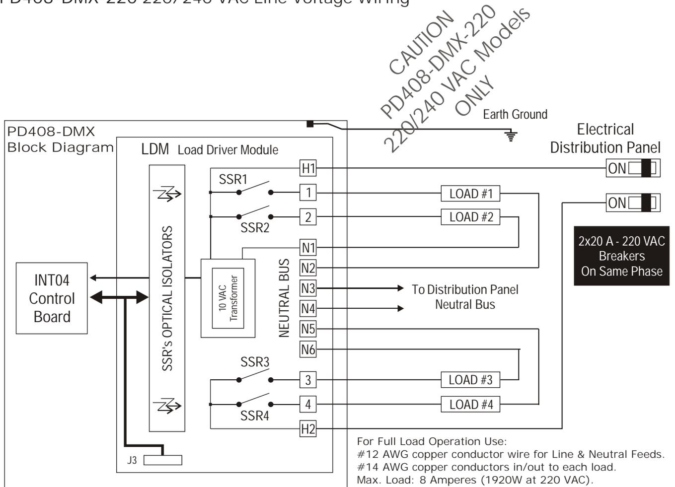
Figure 5. PD408-DMX-220 Typical 220 VAC Wiring.
