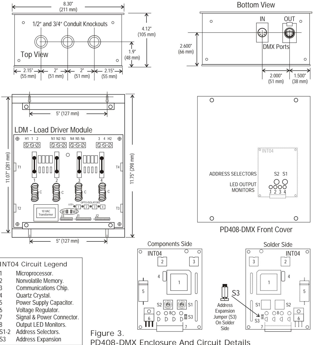
Figure 3. PD408-DMX Enclosure And Circuit Details
