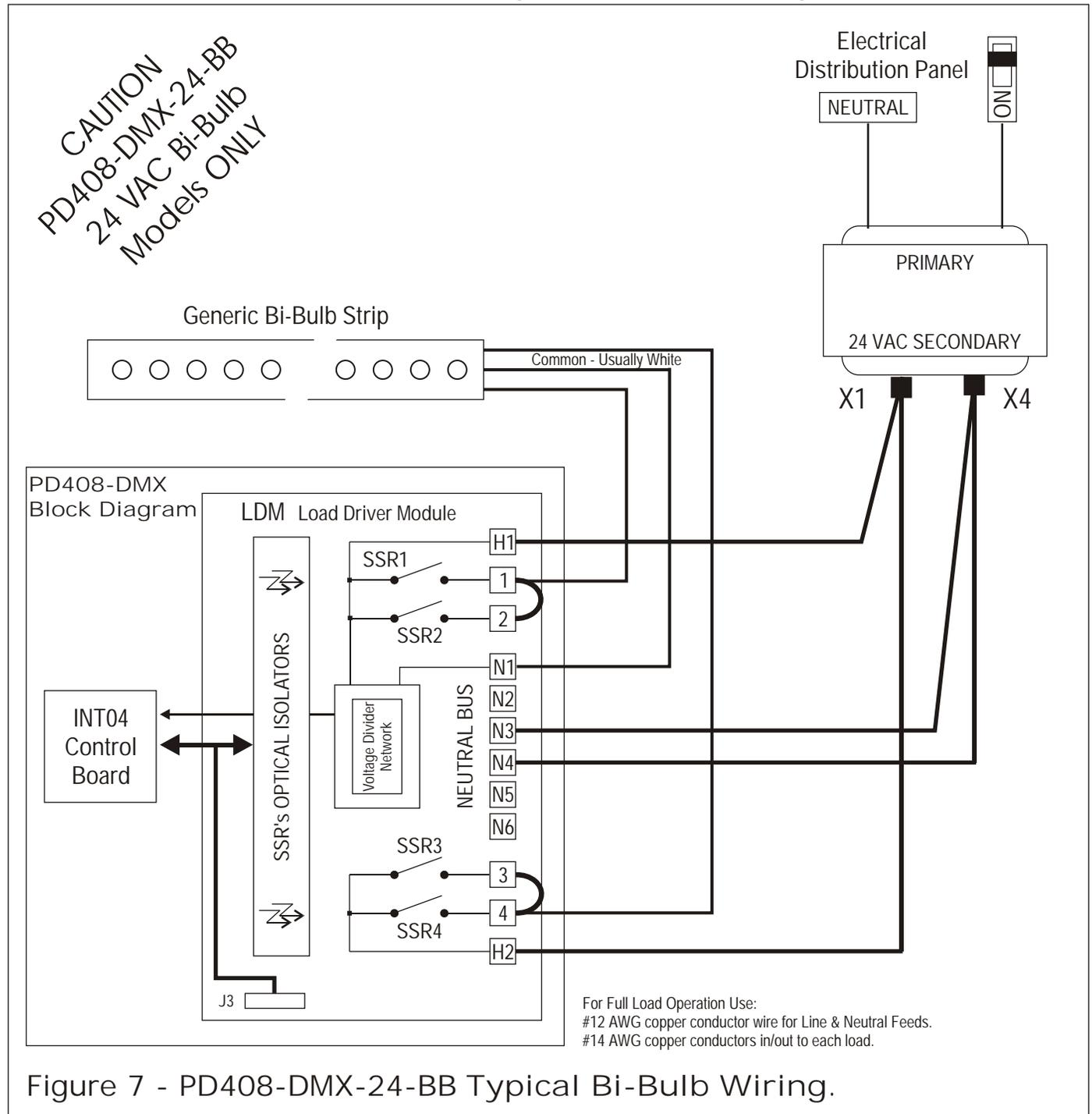
Figure 7 - PD408-DMX-24-BB Typical Bi-Bulb Wiring.
