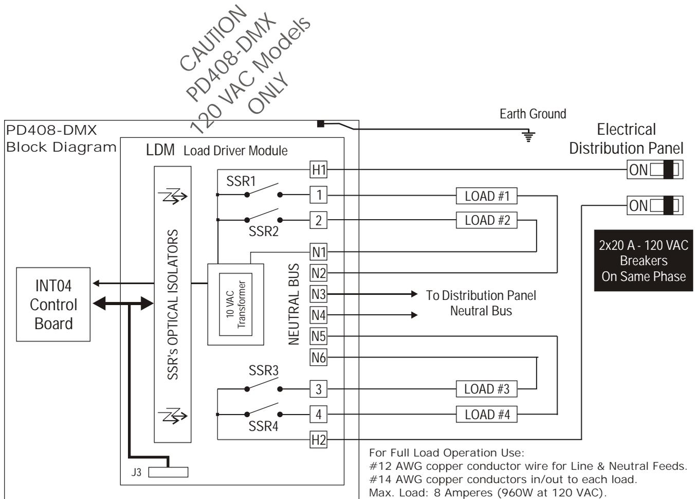
Figure 4. PD408-DMX Typical 120 VAC Wiring.
