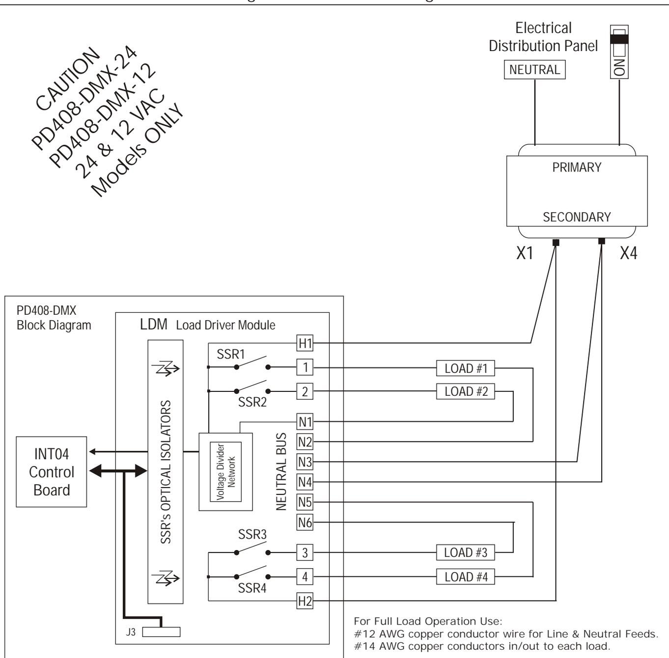
Figure 6 - PD408-DMX-12/24 Typical Low Voltage Wiring.
