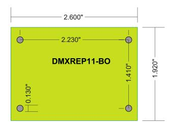
PC board dimensions and mounting holes compatible with **PACTEC** outdoor box model # **OD33-2.0**
