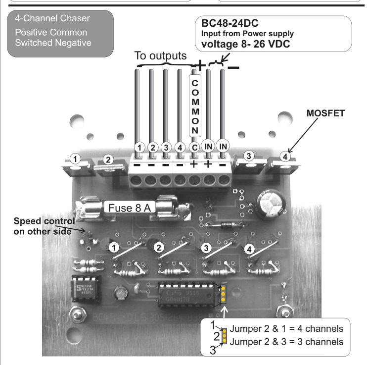
For 4 channel operation Place Jumper between 2 & 1 For 3 channel operation Place Jumper between 2 & 3
