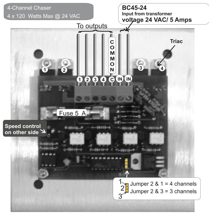
For 4 channel operation Place Jumper between 2 & 1 For 3 channel operation Place Jumper between 2 & 3
