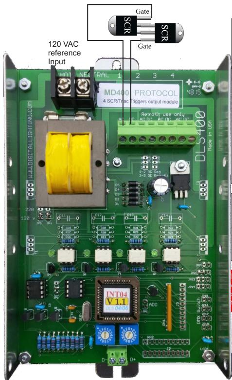
The MD400 Thyristor Firing board is compatible with the PROTOCOL dimming system.
